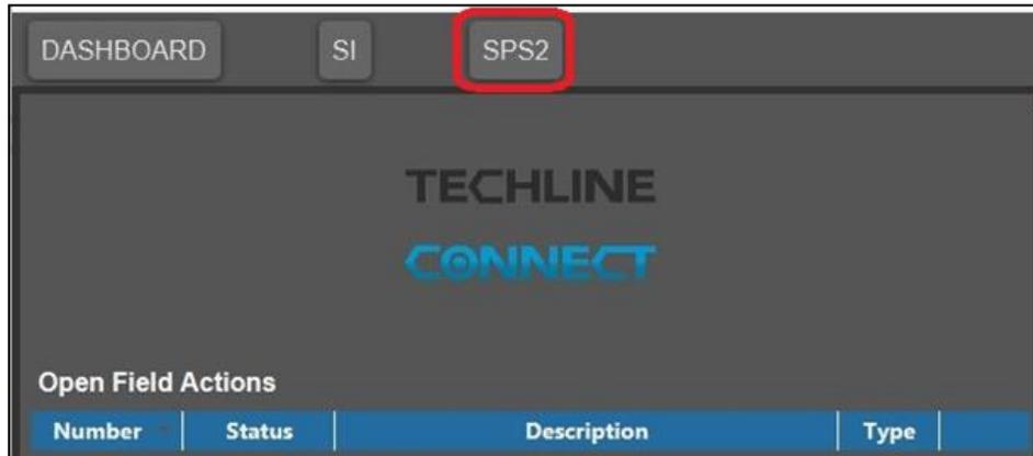
24) SPS2 will open after a short startup and display the detected VIN, there is no need to “build the vehicle”.
